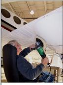
Step 4-B Polish & Seal Wings: Using an adjustable chair, buff the bottom of the wings from the outside bottom tip to the fuselage. The chair allows for a comfortable position when working above your head. Use caution when working in chairs, they tip over easily when the wheels come in contact with air hoses, electrical cords, floor drains, etc... Once both wings are completed, you will have successfully polished and sealed the wings of the aircraft.
