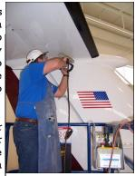
Step 3, Polish & Seal Tail: The tail of the aircraft consists of the vertical and horizontal control surfaces. On the King Air 200, it is necessary to use a scissor lift to reach the tail surface with a buffer. When using a scissor, lift it will be necessary to position the lift within inches of the aircraft. To perform this task safely requires a spotter on the ground. Always clear the aircraft before moving up or down in the scissor lift. Buff top and bottom of the
